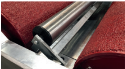
Sensory rollers of stainless steel
