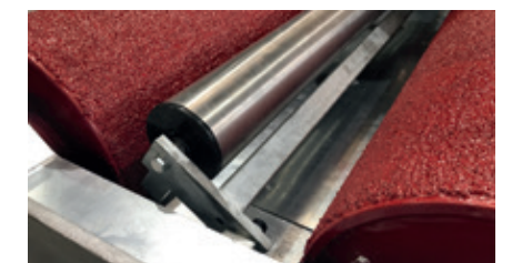
Sensory rollers of stainless steel
