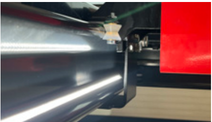
Roller suspensions for scissor jack on the inside of the platform profile
