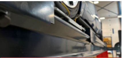
Bended profile for high platform stability
