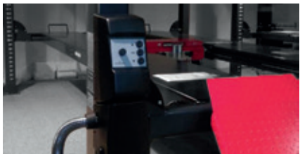
Control unit and power pack on rear left post
