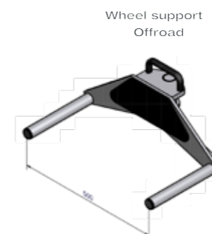
Transporter safely lifted at the wheels
