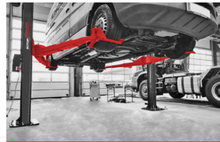
Transporter safely lifted at the wheels
