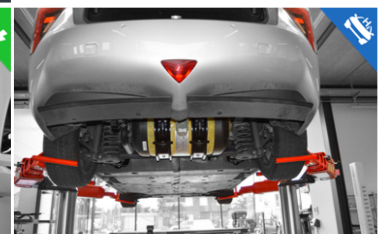
Hydrogen vehicle: Free access to the underbody
